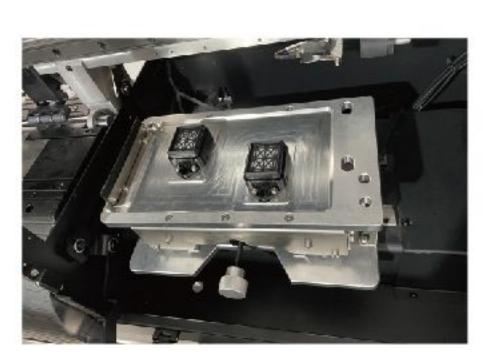
Heating of the printer carriage bottom plate to effectively improve printing stability
