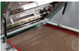
The upper and lower double rows of high - efficiency heating lamps , combined with a unique intelligent heating solution , can save 30% of power consumption
